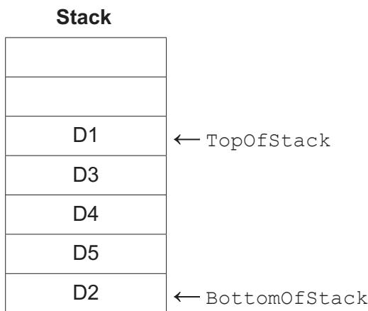
(a) The stack is implemented using two variables and a 1D array of 8 elements as shown.
